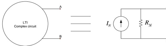
**Figure 5:** Norton Equivalent Circuit
