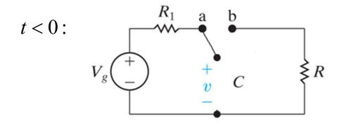
There is an open circuit here, so the current in this circuit is 0, and the voltage drop across  $R_1$  is 0. Thus,
