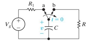
The problem: Find v(t) for  $t \ge 0$ . Note that the circuit to the left of the capacitor establishes an initial voltage drop v(0) across C at t = 0.
