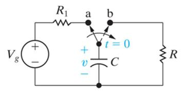
To evaluate the voltage drop across the capacitor for t < 0, put the switch in the "a" position and replace the capacitor with an open circuit. The voltage drop across the open circuit, positive at the top, is
